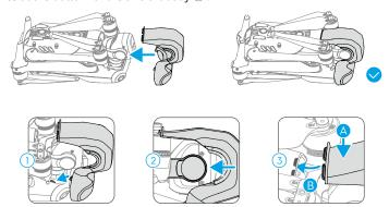
· Make sure to place the propellers of the front arms into the two dents on both sides of the aircraft back. DO NOT push the propeller blades onto the back of the aircraft, which may cause the propeller blades to deform.
