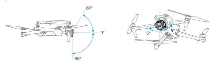
Use the gimbal dial on the remote controller to control the tilt of the gimbal. Alternatively, do so through the camera view in DJI Fly. Press and hold the screen until the gimbal adjustment bar appears. Drag the bar up or down to control the tilt and left or right to control the pan.
