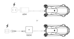
b. If connecting the DJI 100W USB-C Power Adapter to the DJI Air 3 Battery Charging Hub, it takes approximately 1 hour to fully charge an Intelligent Flight Battery inserted into the charging hub.
