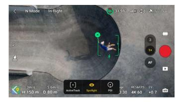
b. Tap on the bottom of the screen to switch to Point of Interest. After setting the flight direction and speed, tap GO and the aircraft will automatically start circling around the subject at the current altitude. The user can also move the control sticks to manually control the flight while the aircraft is automatically flying. Tap the shutter/record button on the camera view in DJI Fly or press the shutter/record button on the remote controller to start shooting.
