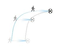
↑ In Trace mode, the direction setting is only effective when the subject is moving in a stable direction. If the moving direction of the subject is not stable, the aircraft will track the subject from a certain distance and altitude. Once the tracking starts, the direction of tracking can be adjusted through the direction wheel.
