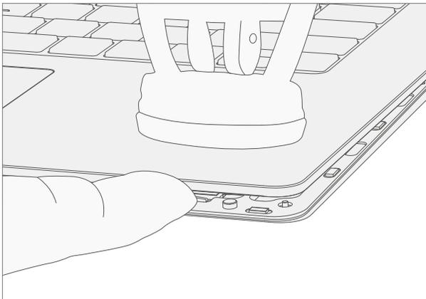
5. **Angle C-cover** – Angle the C-cover at approximately 45 degrees from horizontal – be sure to angle the keyboard **no more than 45 degrees** or else risk damaging the keyboard hook or FPC. If hook is damaged, it needs to be removed carefully to avoid damaging the FPCs, and then a new keyboard needs to be installed.
