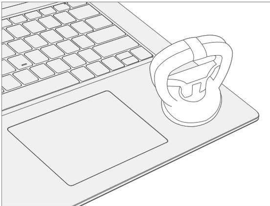
4. **Separate keyboard from device** – Once keyboard separation from the device bottom case is achieved, place a finger between the keyboard and device region. Pull upwards slightly to separate the keyboard from the magnets.
