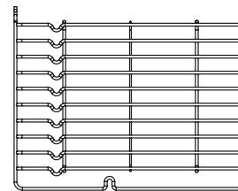
**Telescopic runner:** Some models might with telescopic runners to facilitate the use of oven. These telescopic runners and slider brackets could be disassembled by unscrewing the screws used to fix it. After disassembled, dishes and tray can be put on the oven floor, using functions as Radiant grilling, Double grilling, Double grill with fan.
