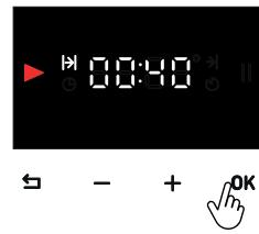
with **OK** button, move forward until the screen above appears and start the cooking.
