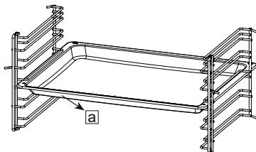
Accessories should be placed between two racks and the side with a inclination should face the door of the appliance.
