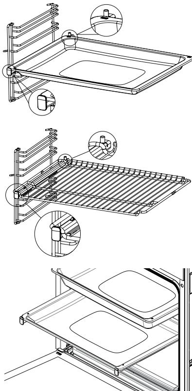
Push the rails completely inside without placing the tray and wire grid on them. Accessories must be between the front and rear overhangs of the rails.
