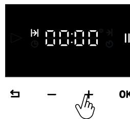
Firstly, select the minute with **- +** buttons and activate the clock by pressing on **OK** button.
