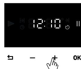
Firstly, select the minute with - + buttons, by pressing on **OK** button, select the hour and confirm it with **OK** button.
