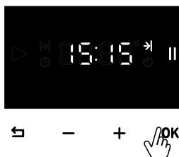
For cooking completion, after selecting the minute and the hour, move forward with **OK** button until the cooking screen appears.
