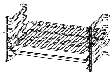
You can use the tray as a drip tray for grilled food and meat dishes by placing the tray and the rack together.
