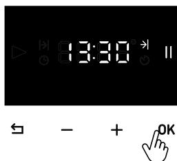
For cooking completion, after selecting the minute and the hour, move forward with **OK** button until the cooking screen appears.
