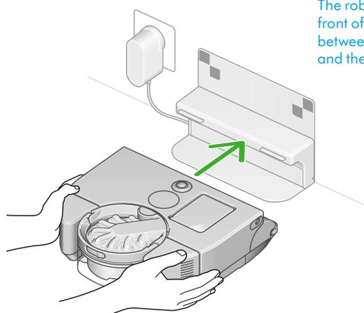
The robot sits in the front of the dock between the floor plate and the front ridge.
