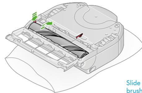
Slide and lift the brush bar out from one end and remove whole component
