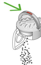
With the handle lifted, the cyclone release button is located in the middle of the handle.
