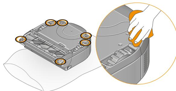
Locate seven sensors on the base of the machine. Two sensors on either side towards the rear. Two are located on the front corners. One sensor is located in the recess in front of the right wheel.
