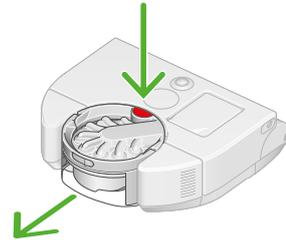
The bin removal catch is located behind the screen on the top of the robot. This can be pressed and the bin pulled away from the main body.
